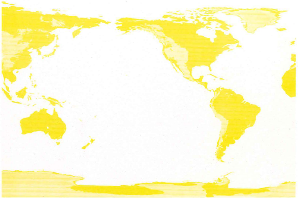
Photo 5. World Topographic Map (Progressive plate for yellow) Platemaking by using Colour Electrostatic Plotter : Adopted data...ETOPO 5 (NOAA, U. S. A.)
