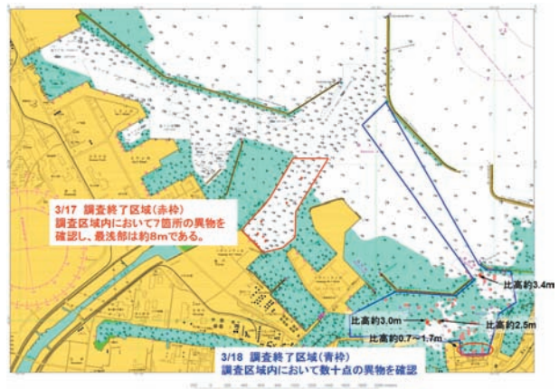
図3 八戸港調査実施区域と異物の位置。 Fig.3 Map of the area surveyed in Hachinohe port and the locations of detected obstructions (red dots).
