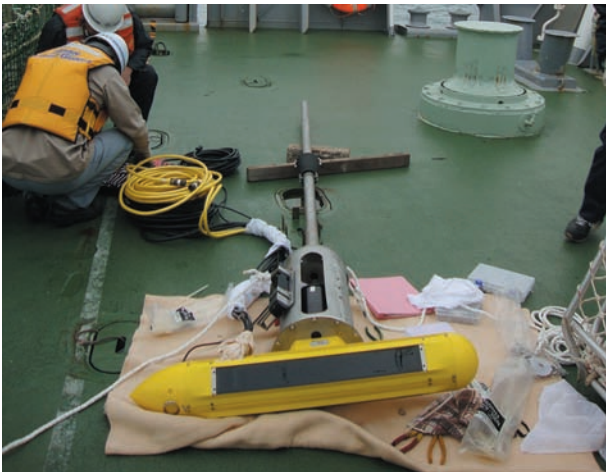
写真 26 C3D-LPM 送受波器。 Photo 26 C3D-LPM sonar head.
