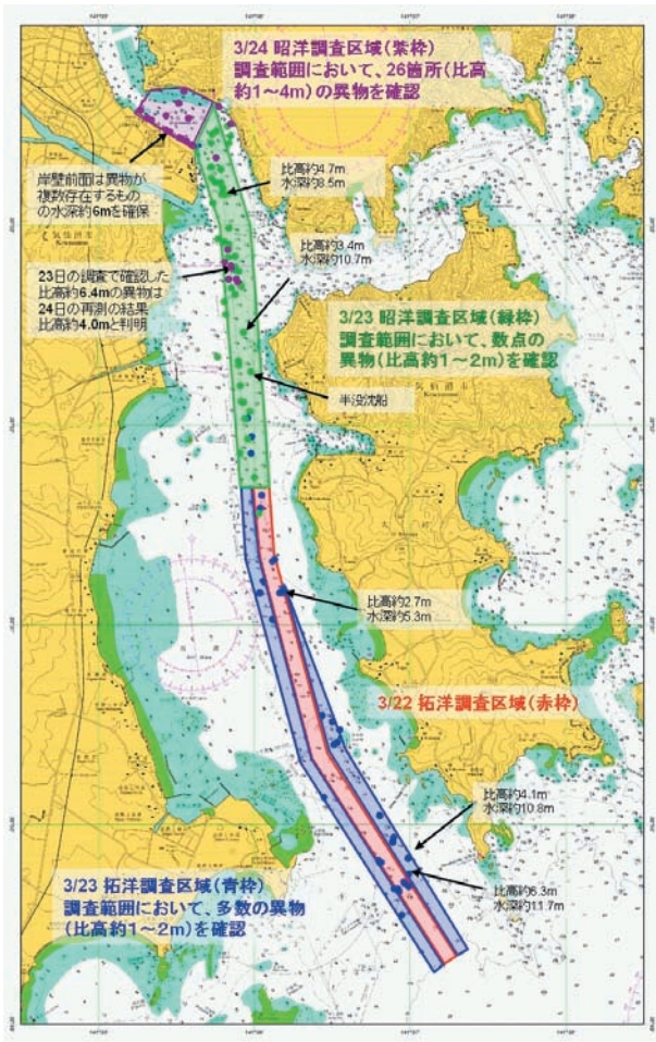
図8 気仙沼港調査実施区域と異物の位置。 Fig.8 Map of the survey area in Kesennuma Bay showing the location of detected obstructions.
