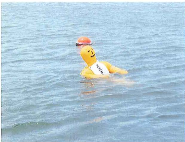
写真3 漂流実験用人形と漂流ブイ Photo.3 Puppet for drift experiment, and drifting buoy.
