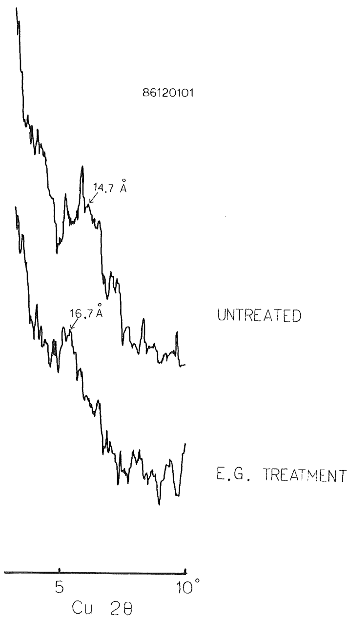
Figure 4-1b Low angle X-ray diffraction figures of the untreated sample and the ethylene glycol treatment sample
